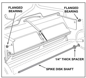
• Place a short spacer tube, a drive disk, a 5/8" flat washer, another drive disk and a second 5/8" flat washer onto the shaft. Fit the short spacer tube onto the flanged bearing in the end plate. See figure 14.
